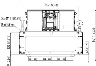
**Heating Capacity** 14.8kW – 50499 BTU/hr
