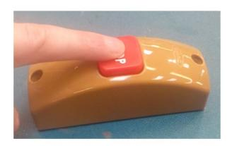
Press the Bell Push button. *This must* be done within 30 seconds of CH0 starting to flash CH0 should remain on steady for approximately 4 seconds
