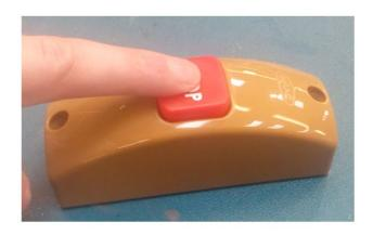
Press the Bell Push button. *This must be* done within 30 seconds of CH2 starting to flash CH2 should remain on steady for approximately 4 seconds
