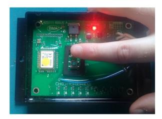
Press and hold the Clear Button on the receiver until the Learn Mode Indicator lights and CHO starts to flash.
