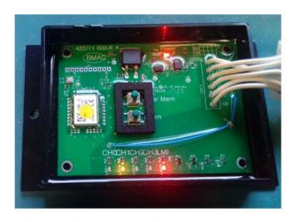
CHO Indicator should start flashing. Press the Learn Button again, CH1 should start flashing
