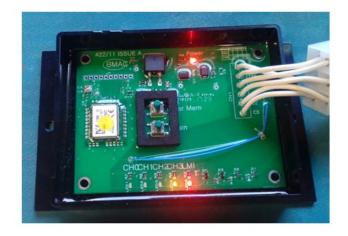
CHO Indicator should start flashing. Press the Learn Button twice to cycle through CH1 & CH2. CH3 should start to flash
