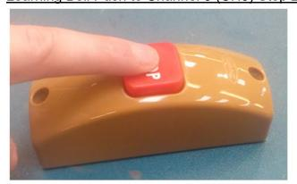
Press the Bell Push button. *This must be done within 30 seconds of CH3 starting to flash* CH3 should remain on steady for approximately 4 seconds
