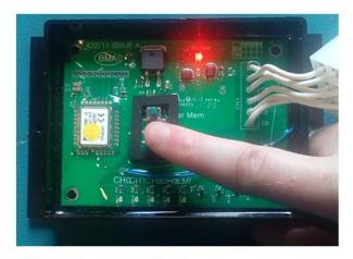
Press the Learn Button three times to Cycle through CH1, CH2 & CH3. The Learn Indicator will switch off. All programmed Bell Pushes to the receiver will be cleared.
