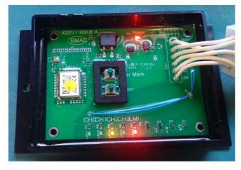
CHO Indicator should start flashing. Press the Learn Button twice to cycle through CH1. CH2 should start to flash.
